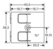
Mounting hole diameter: 3,5 mm
