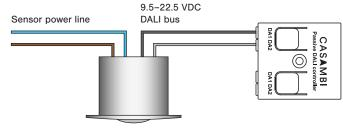
Sensor with integrated DALI power supply
