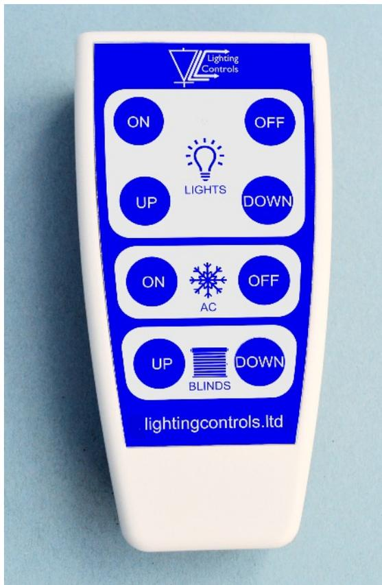
The **ecoLUX** PIR Remote Control is highly flexible and communicates with the lighting control network through a PIR. Upto 8 buttons can be configured to do any control task that can be performed by the PIR from scene changes, over rides or dimming, to heating or window blinds.
