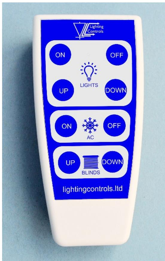
The **ecoLUX** 'Hand held Scene Plate' remote performs the functions of a scene set control plate. This is used with our plug in and hardwired control modules to control different lighting groups at different levels as well as some other non-lighting functions, such as electric blinds.
