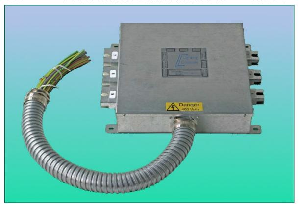
The ecoFLEX 9 Port Master Distribution Box is supplied pre-wired with a home run cable containing up to nine circuits of LSOH cable. The system can also incorporate selected bus cables for a fully integrated lighting and controls wiring solution.
