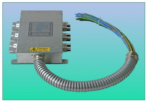
The ecoFLEX 6 Port Master Distribution Box is supplied pre-wired with a home run cable containing up to nine circuits of LSOH cable. The system can also incorporate selected bus cables for a fully integrated lighting and controls wiring solution.
