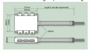
Metal Housings: Bright Spangled Galv - BSEN10142:2000 Protection Class: IP20 Conduit: Galv - BSEN50086 Current rating: 25A Voltage rating: 400V/6kV/3.IEC60664
